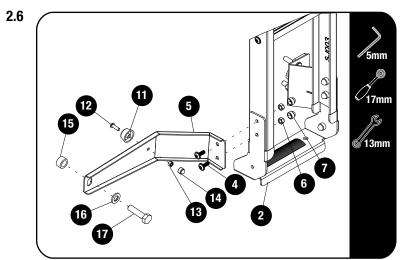
Assemble the Spare Wheel Mounting
