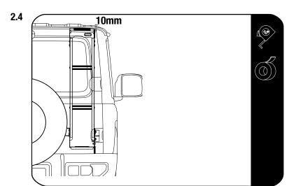
Place the U-Channel Rubber (Item 10) over the door edge where the Top Step Plate (Item 4) will be secured.
