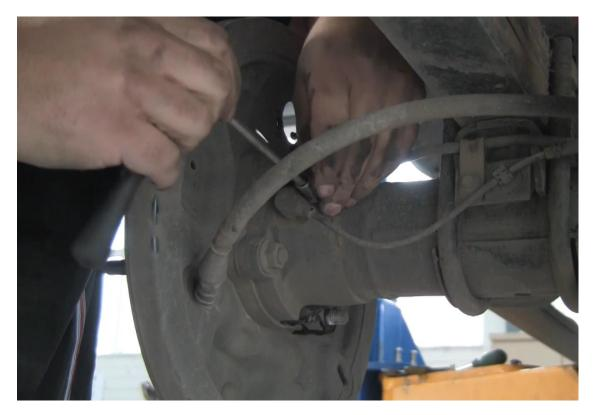
Remove the handbrake retaining clip and cable.
