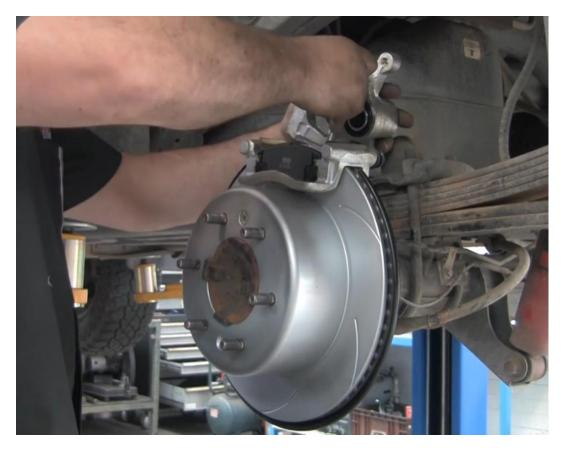
Recheck all bolts are to the correct torque.
