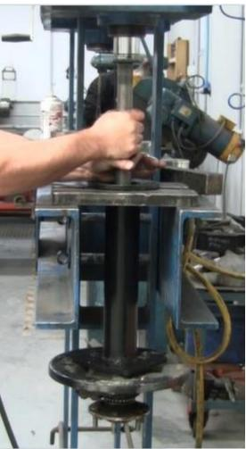
Then remove the bearing from the housing.
