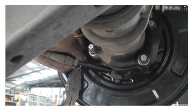
Refit the brake line to the new mount. #15
