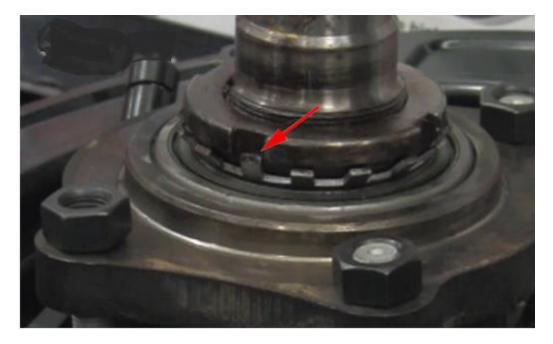
When the locking nut is in place, bend the tab to lock it in place.
