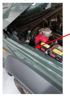
Remove standard M6 bolt from vehicle panel using a 10mm Spanner / Wrench / Socket
