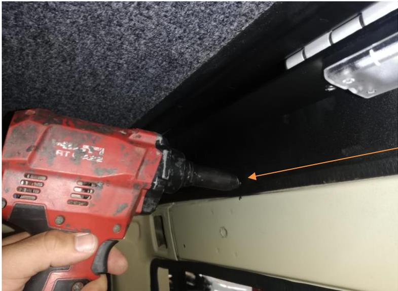
Use a pop rivet gun to secure the pop rivets in place.
