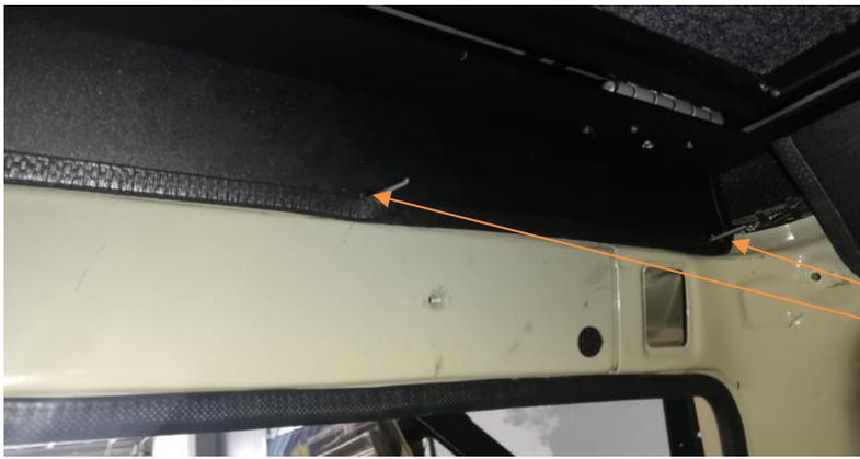
Once the holes have been drilled bigger, you can now proceed to fit the rear panel in place and insert the pop rivets
