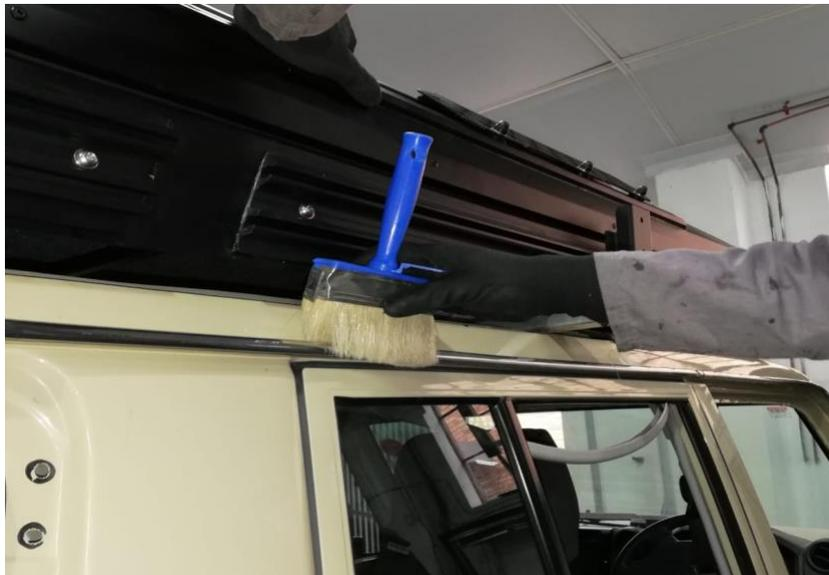
You can now apply the Sika flex to the vehicle all along the sides and rear, as seen below.
