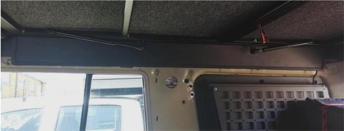
The rear panel should be fitted roughly into place and with a marker, the holes on the body that correspond with the cover plate should be marked out and drilled to 5mm in diameter.
