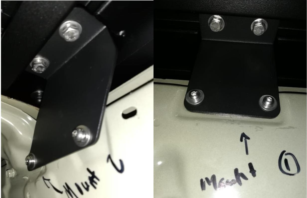
Once the Roof conversion is bolted down, you may now proceed to seal the sides and all around the roof as seen below with the appropriate colour sealant. (Please note that the images below are for reference purposes and are similar to the Thor roof conversion but not exactly the same).
