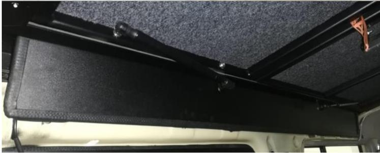
Cover Panel in place. (Note: the picture displayed here shows the large and small bed sections in the closed position, however the bed sections will need to be in the open position in order to pop in the rivets)
