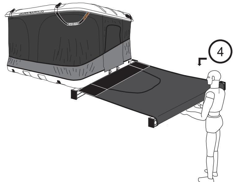
⑯ Unwrap the strips fixing the awning and unroll it. Remove both telescopic legs and place them on the ground. Lock them at the desired height, turning them in the direction as shown. Repeat the same operation with the horizontal tubes, fitting them in their assign locations and lock them by giving the correct tension to the awning.
