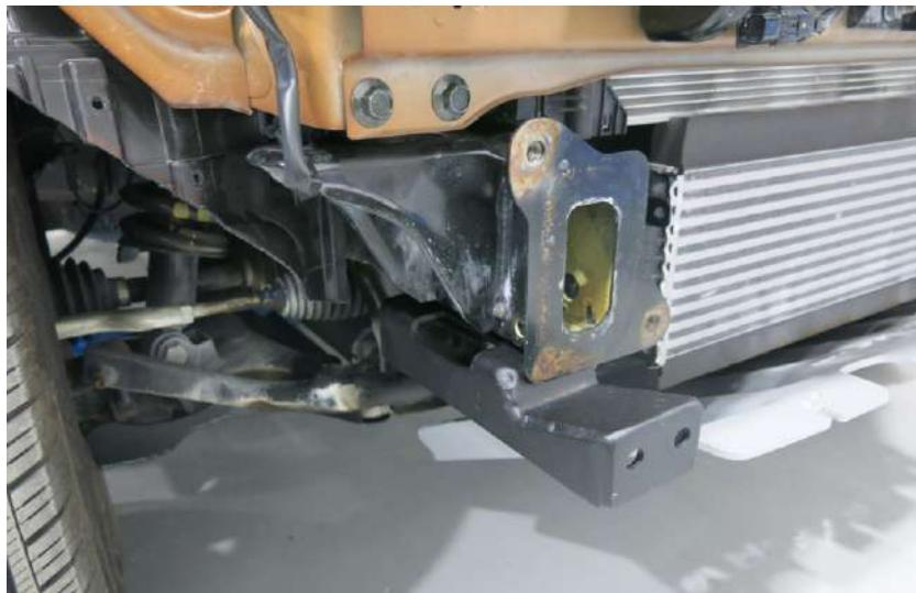
23. Install right frame booster (pos. 3) onto the vehicle frame, secure with standard bolts with installation of standard towing eye. Do not tighten screw joints.
