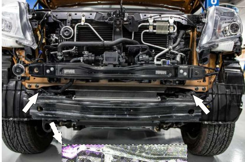
19. Unscrew 4 tension bolts of the frame booster. Dismantle the booster.
