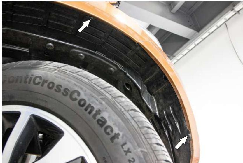
8. Unscrew 2 self-tapping screws of the bumper clamp in arches on the left and right.
