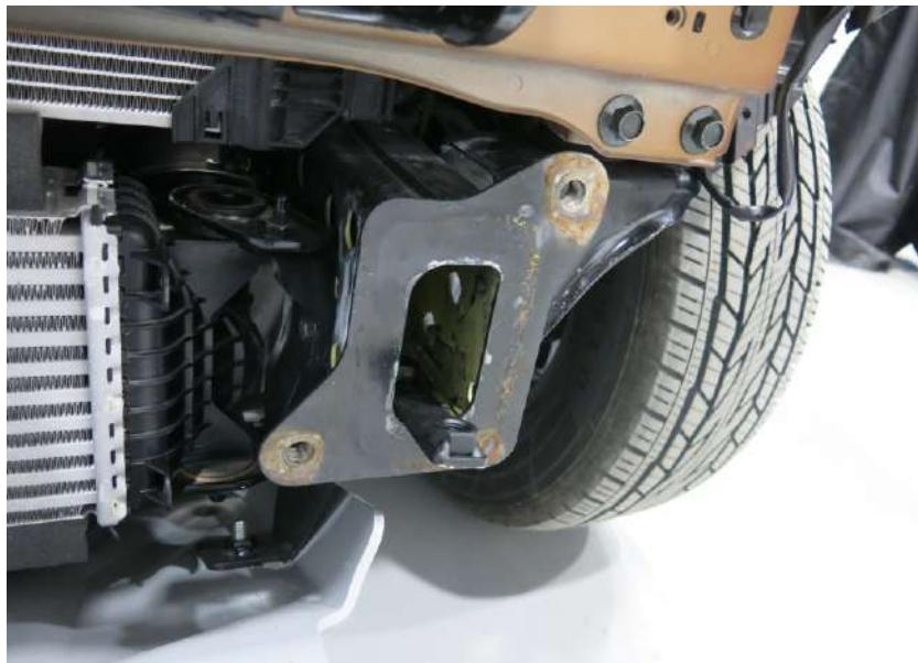
21. Insert embedded part M12 (pos. 8) into the frame on the left.
