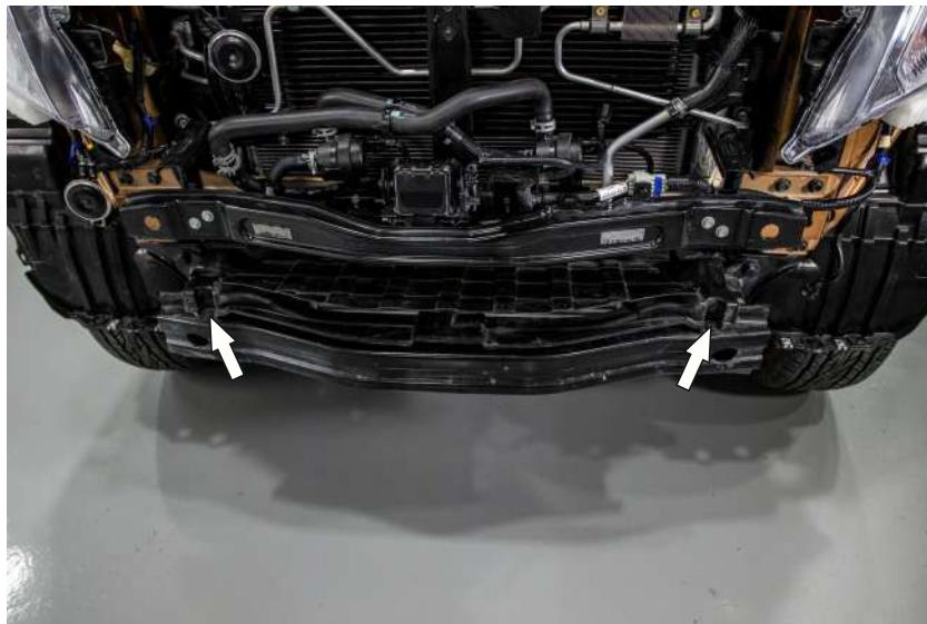
18. Remove the air intake clips. Dismantle the air intake.
