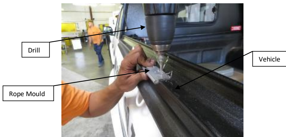
Figure 5: Drilling Mounting Holes into vehicle
