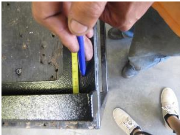
Figure 19: Measuring mounting holes on the frame
